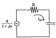
Also sketch the amplitude and phase spectrum. If the above voltage is applied across a series RC circuit, find i(t).
