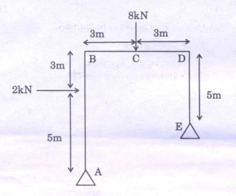
12. (a) Analyse a frame shown below using Cantileverl method. Draw also the BMD.
