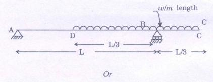
12. Determine the rotation at A and deflection at C in the overhanging beam shown in fig. below:
