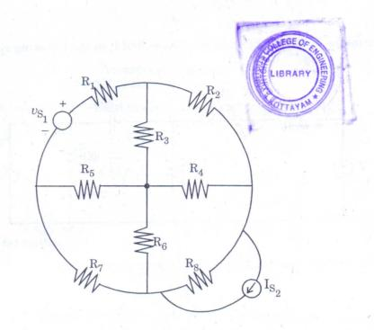
For the above network, draw the system graph. Select a tree and perform cut-set schedule. Also calculate all branch voltages and branch currents.
