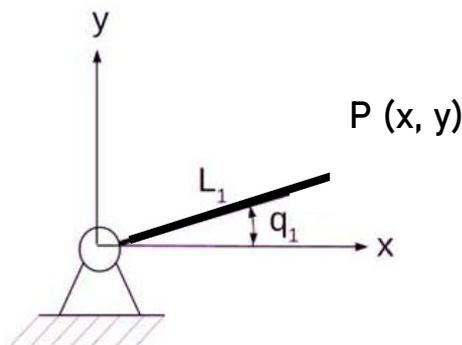
Calculate the torque of a 1 degree of freedom serial manipulator using Lagrange's Equation  $T = \frac{d}{dt} \left( \frac{\partial L}{\partial \dot{q}_i} \right) - \frac{\partial L}{\partial q_i}$ , where L is the lagrangian. Take mass of the link as m and Inertia as that of a rectangular section. Take appropriate notations for any missing parameters.
