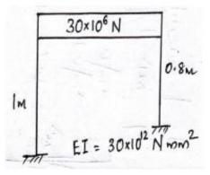
13. Find the response for an damped system subjected to the loading as shown
