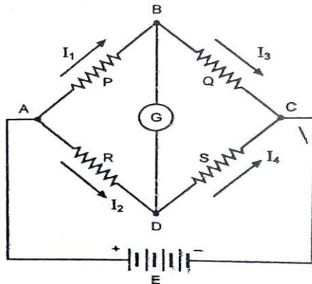
The Wheatstone bridge shown when used for determining the value of unknown resistance  $R$ , is balanced when  $P=100\ \Omega$ ,  $Q=10\ \Omega$  and  $S=46\ \Omega$ . Determine the value of unknown resistance.
