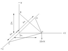
11 a) Find the reactions at the supports A(hinged) and B (roller).
