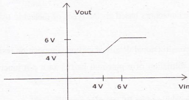
15. Assuming drop across diode is 0.6V, find output voltage  $V_0$ ?
