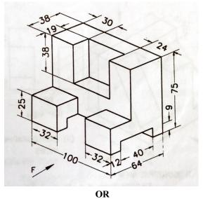
10. Draw the top view, front view (take the arrow as reference) and left side view of the object shown below. Any missing dimension may be suitably assumed.
