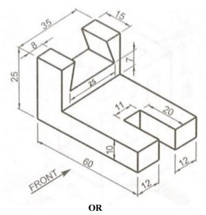
10. Draw the top view, front view and left side view of the object shown below. Any missing dimension 12 may be suitably assumed.
