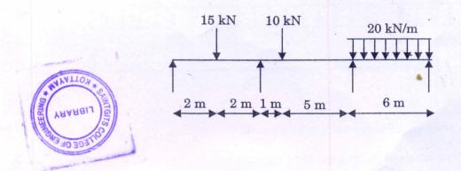
13. Plot B.M.D. and deflected shape of the following structure using slope deflection method.
