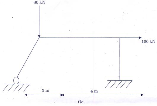
18. A statically indeterminate frame shown in Fig. below. It carries a load of 80 kN. Analyze the frame by matrix flexibility method. A and E are same for all members.
