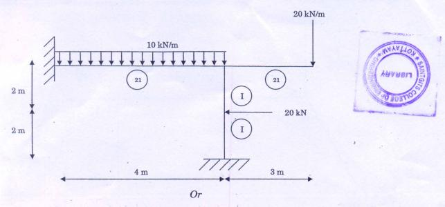
14. Analyze the portal frame loaded as shown in the Fig. below. Use moment distribution and sketch B.M.D. and S.F.D.
