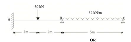
18. Analyse the given frame using direct stiffness matrix method.
