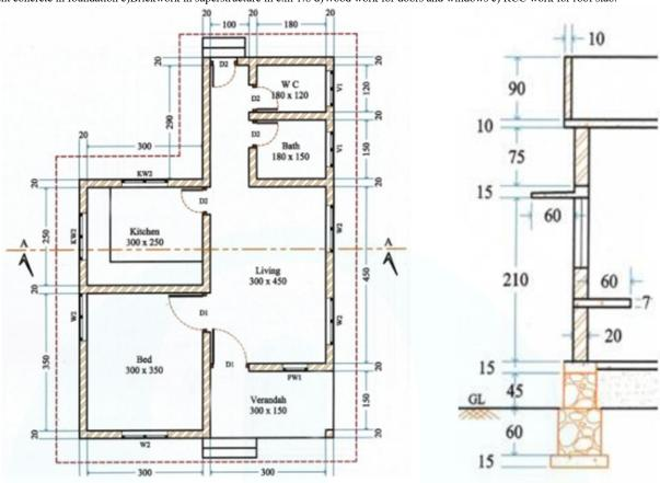
6. Calculate the quantity of RCC work involved in the construction of the slab of size 330 cm x 550 cm (internal dimensions) shown in figure below 25 and prepare a bar bending schedule. All dimensions are in centimetres.
