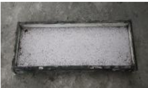
Fig 4. Wooden moulds of dimension 400 \times 100 \times 16 mm
