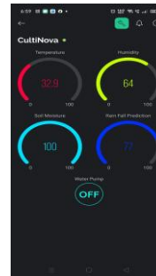
Fig 2: Blynk App Display of Soil Parameters
