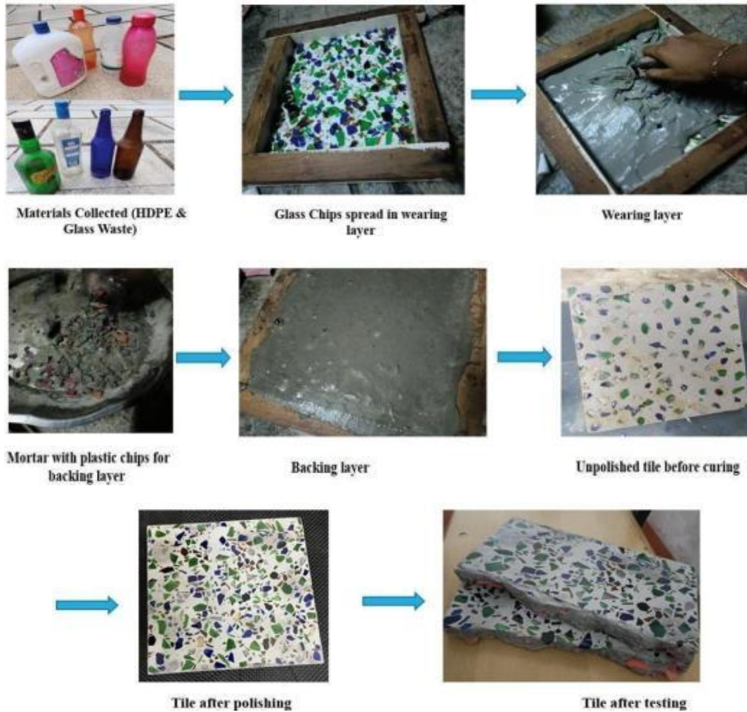
Fig. 1. Process of producing mosaic tiles using waste glass chips and plastic chips
