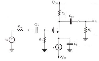
Draw the small signal equivalent circuit of the amplifier shown. Find out its voltage gain and output Impedance.
