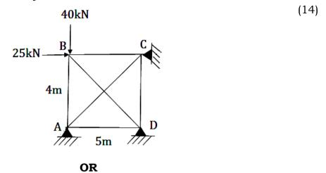
16. Analyse the given frame using displacement transformation matrix
