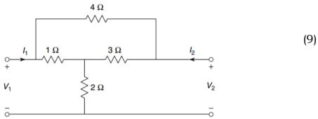
b) Derive the expression for z parameters in a two-port network. (5)
