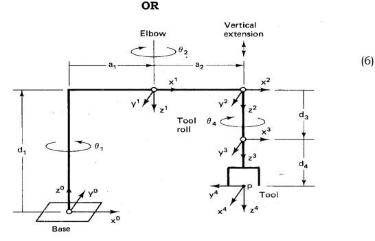
Represent the DH parameters of the given robotic arm. Evaluate the arm matrix.
