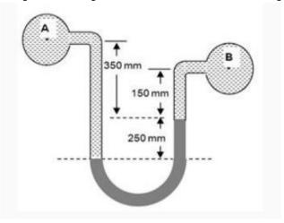
b) A simple U-tube manometer is installed across an orificemeter. The manometer is filled with mercury (sp. gravity = 13.6) and the liquid above the mercury is carbon tetrachloride (sp. gravity = 1.6). The manometer reads 200 (6) mm. What is the pressure difference over the manometer in newtons per square metre.
