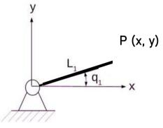
Calculated the torque of a 1 degree of freedom serial manipulator using Lagrange's Equation  $T = \frac{d}{dt} \left( \frac{\partial L}{\partial \dot{q}_i} \right) - \frac{\partial L}{\partial q_i}$ , where L is the lagrangian. Take mass of the link as m and Inertia as that of a rectangular section. Take appropriate notations for any missing parameters.
