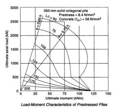
Sectional properties of 35mm solid octagonal pile: A =  $1.02 \times 10^5$  mm<sup>2</sup>, Weight = 2.45 kN/m, Z =  $4.70 \times 10^6$  mm<sup>3</sup>, i = 90 mm
