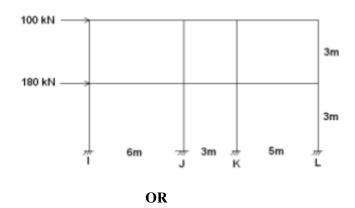
16. Analyze the frame shown in figure using portal method.
