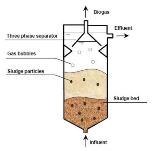
It is somewhat modified version of the contact process, based on an upward movement of the liquid waste through a dense blanket of anaerobic sludge. No inert medium is provided in these systems. The upflow anaerobic sludge blanket reactor (UASB) is a single tank process. Wastewater enters the reactor from the bottom, and flows upward. A suspended sludge blanket filters and treats the wastewater as the wastewater flows through it.
