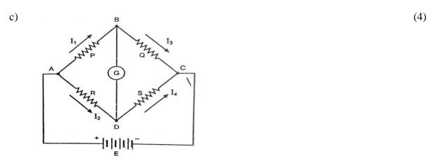
The Wheatstone bridge shown when used for determining the value of unknown resistance R, is balanced when  $P=100 \Omega$ ,  $Q=10\Omega$  and  $S=46 \Omega$ . Determine the value of unknown resistance.
