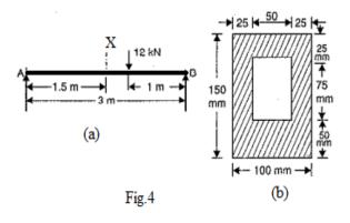
Determine the bending stresses at extreme fibres at section X-X. Take moment of inertia about neutral axis of the section as  $2.56 \times 10^7$  mm<sup>4</sup>.
