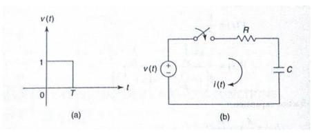
b) For the network shown plot poles and zeros of function  $I_0/I_i$
